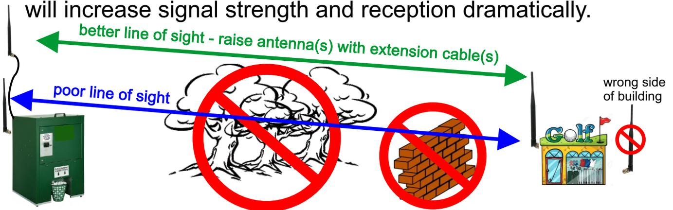
Line of site is best, raise either the ball dispenser antenna or the pro-shop antenna to a higher height, using an optional antenna extension cable if obstructions are present. Obstructions will reduce the distance from over 2000 feet to less than 300. When installing the receiver in the pro-shop, make sure it is in a window that faces the ball dispenser and is as high as possible.
