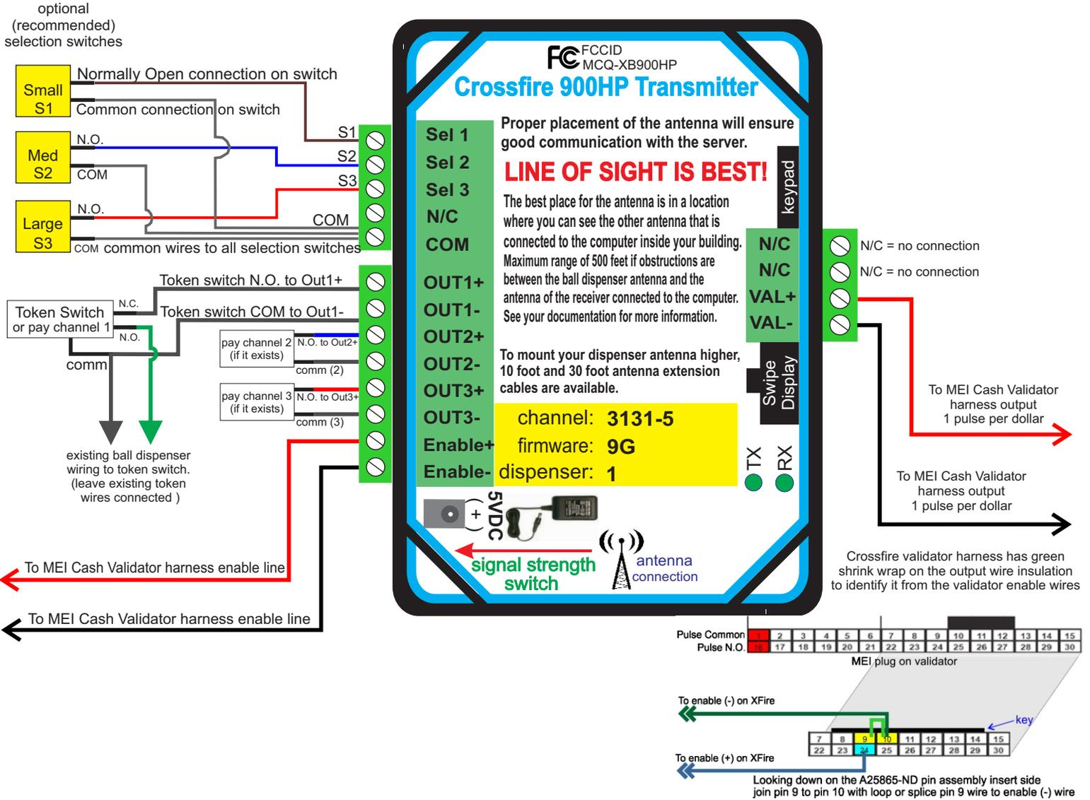
Proper antenna placement with few obstructions will increase signal strength and reception dramatically.
